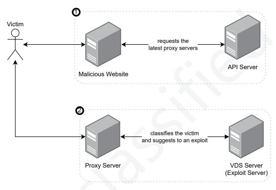
Figure 4. The infrastructure of the RIG exploit kit.
